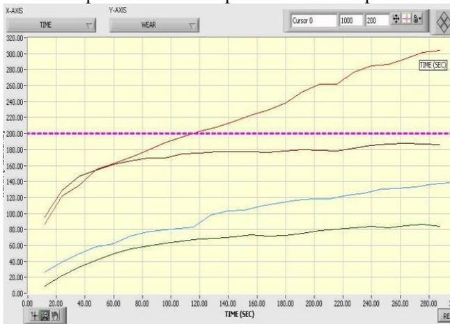
Graph3: shows the wear test of sample 1,2,3,4
