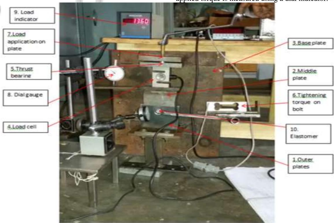
Fig. 1: Experimental set up to evaluate joint stiffness.
