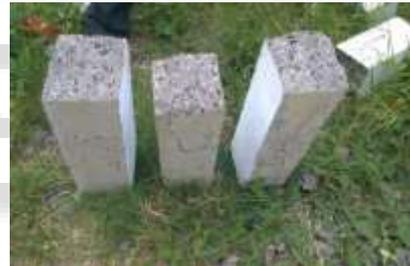
Fig. 3.2(a): The fractured beams of DA type specimen.
