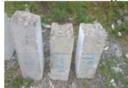
Fig. 3.2(b) The fractured Beams of VB type specimen.
