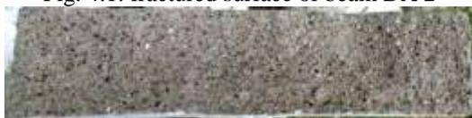
Fig. 4.2: Fractured surface of mortar panel PM 1
