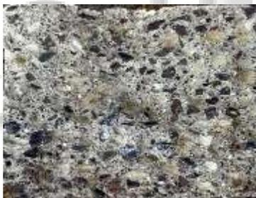
Fig. 4.1: fractured surface of beam DA 2
