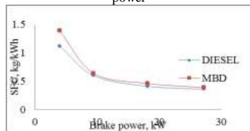
Fig. 12: Variation of specific fuel consumption with brake power
