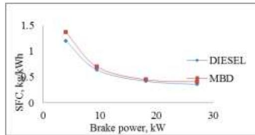
Fig. 19: Variation of specific fuel consumption with brake power
