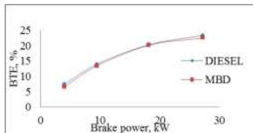
Fig. 11: Variation of brake thermal efficiency with brake power
