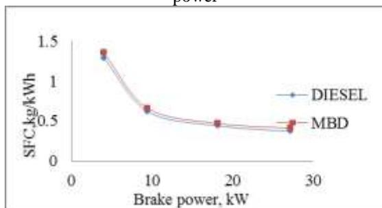
Fig. 5: Variation of specific fuel consumption with brake power
