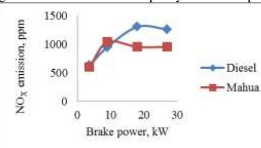
Fig. 24: Variation of NO<sub>x</sub> with brake power
