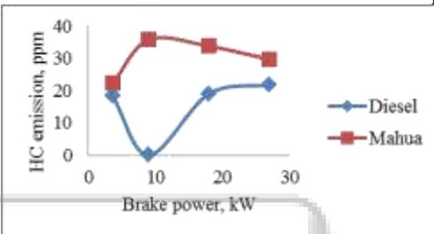
Fig. 15: Variation of unburnt hydrocarbon with brake power
