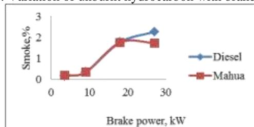
Fig. 9: Variation of smoke opacity with brake power
