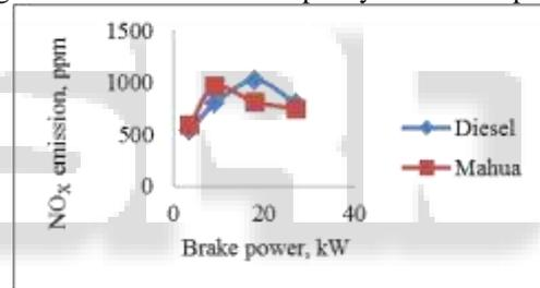
Fig. 10: Variation of NO<sub>x</sub> with brake power
