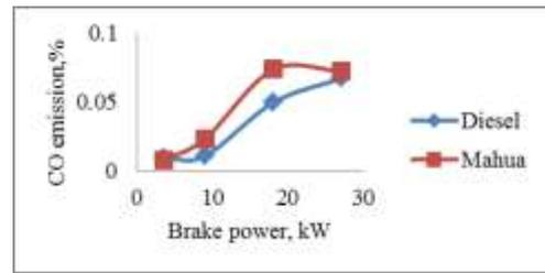
Fig. 7: Variation of carbon monoxide with brake power
