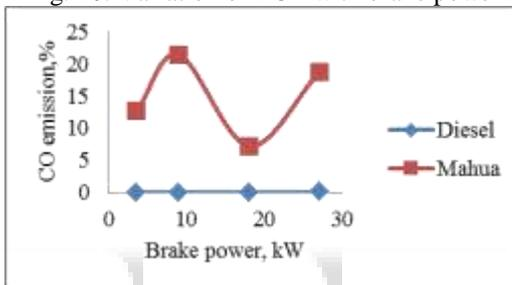
Fig. 21: Variation of carbon monoxide with brake power
