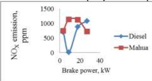
Fig. 17: Variation of NO<sub>x</sub> with brake power
