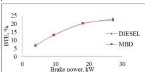
Fig. 18: Variation of brake thermal efficiency with brake power
