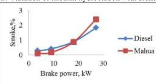
Fig. 23: Variation of smoke opacity with brake power
