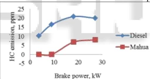
Fig. 22: Variation of unburnt hydrocarbon with brake power
