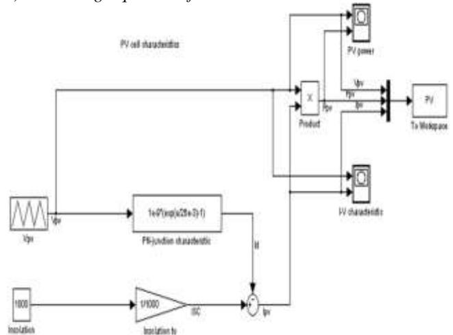
Fig. 4: Modeling Equation of Solar Cell
