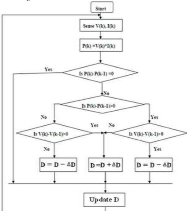
15) Photovoltaic System using with MPPT Technique
