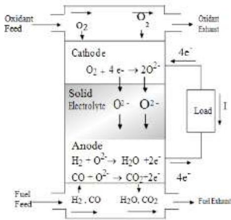
Fig. 13: Basic Electrochemistry of an SOFC
