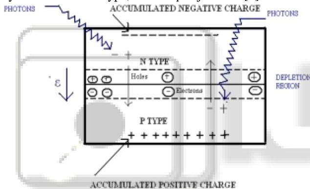
Fig. 3: Illustration of the p-n junction of PV cell showing hole-electron created by photons
