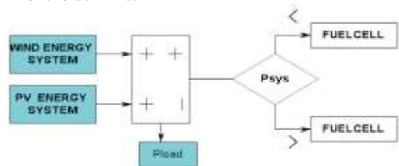
Fig. 2: Overall Power Management Strategy for the Hybrid Energy Generation System
