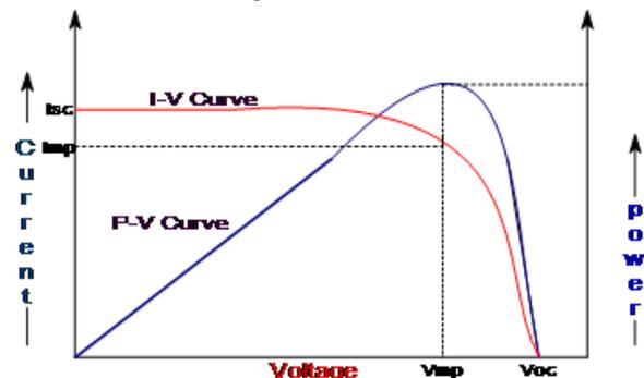
Fig. 7: V-I & P-V curve for PV cell
