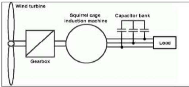
Fig. 10: squirrel cage induction generator (SCIG)
