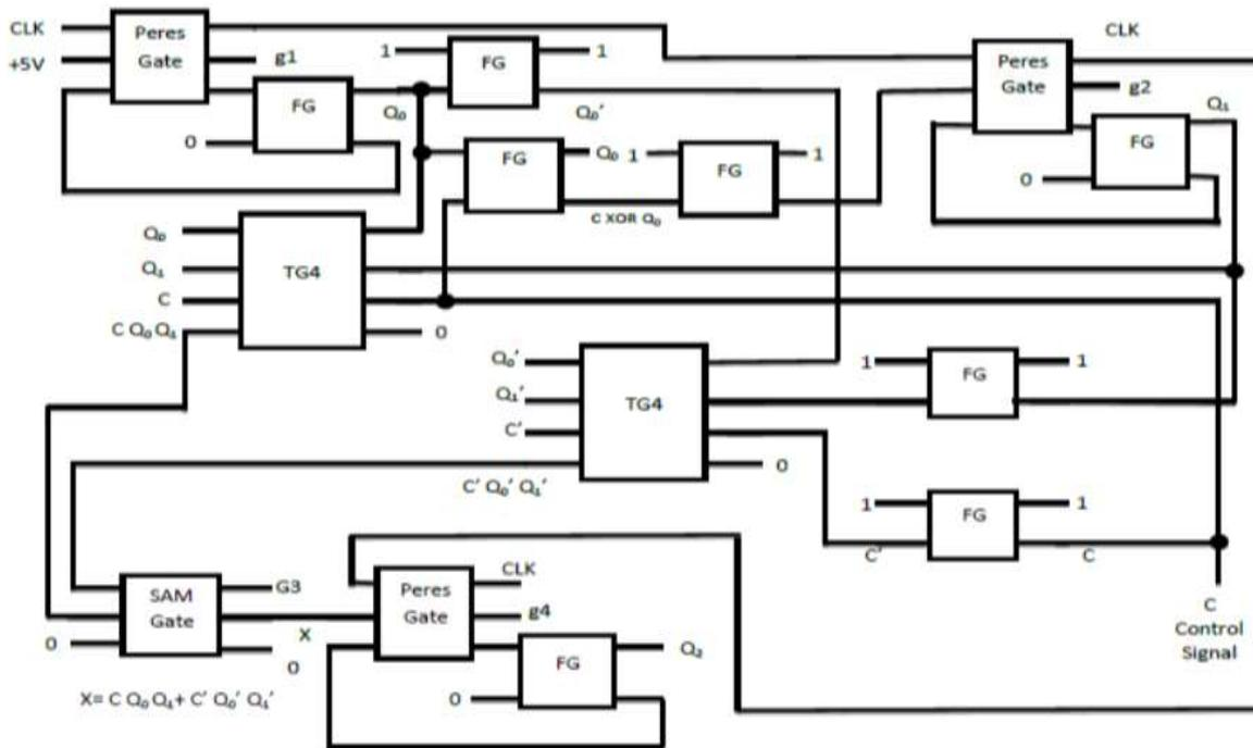
Fig. 9: Proposed Design of MOD-8 Synchronous Up/Down Counter
