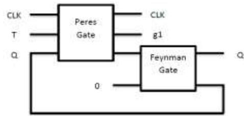
Fig. 6: T Flip-Flop using Peres and Feynman gate
