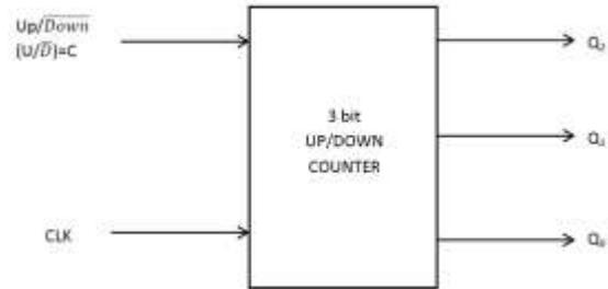
Fig. 7: Block diagram of 3-bit Up/Down counter
