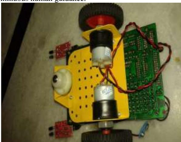
Fig. 1: Obstacle Robot Motor and Sensors
