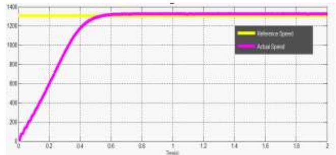
Fig. 9: Actual and Reference Speed Obtained at Loaded Condition
