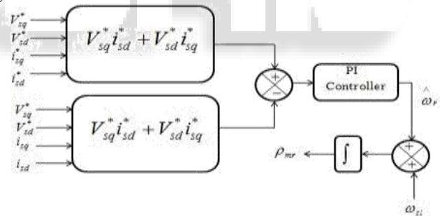
Fig. 1: Block Diagram of Speed Estimation
