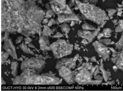
Fig. 13: SEM image of concrete with WA 10% replacement at 28 days
