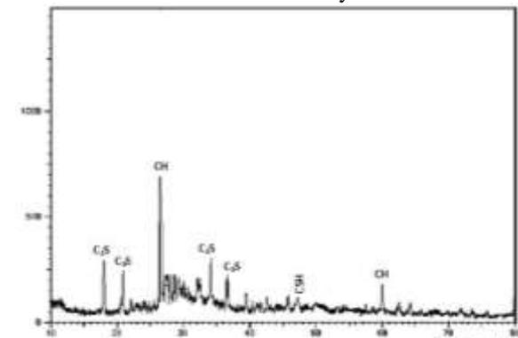
Fig. 5: XRD pattern of cement mortar (1:3) with 30% WA addition at 28 days
