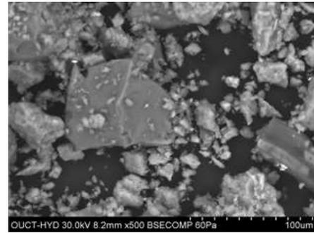
Fig. 17: SEM image of concrete with WA 30% replacement at 28 days
