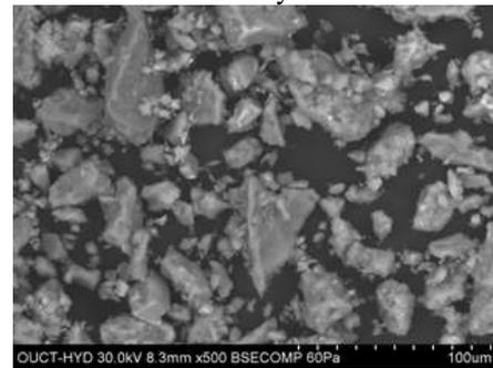
Fig. 20: SEM image of concrete with WA 30% addition at 90 days
