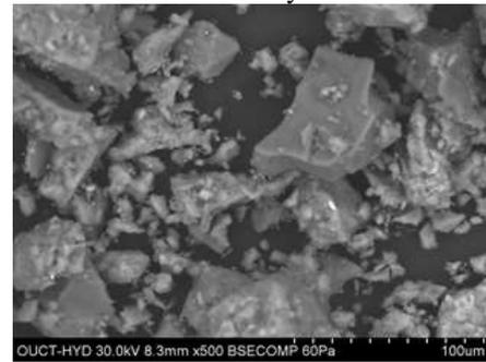
Fig. 18: SEM image of concrete with WA 30% replacement at 90 days
