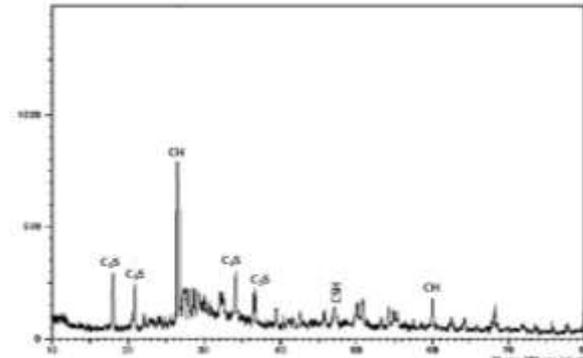
Fig. 3: XRD pattern of cement mortar (1:3) with 30% WA replacement at 28 days
