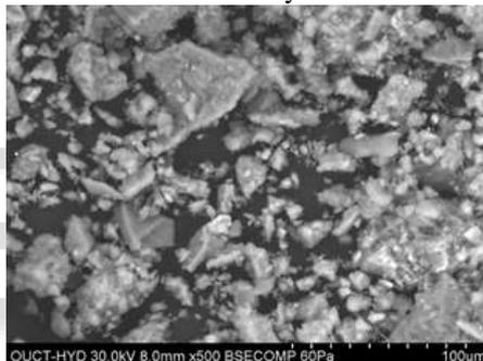
Fig. 19: SEM image of concrete with WA 30% addition at 28 days
