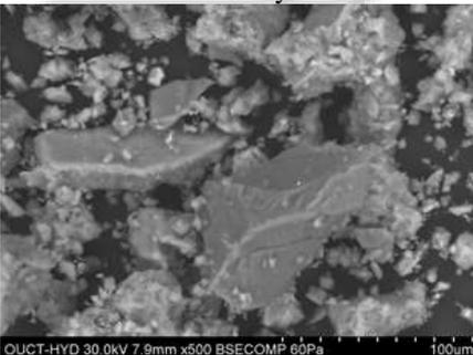
Fig. 15: SEM image of concrete with WA 10% addition at 28 days
