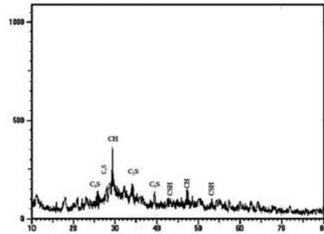
Fig. 10: XRD pattern of cement mortar (1:6) with 30% WA addition at 28 days
