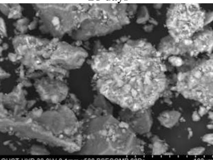
Fig. 16: SEM image of concrete with WA 10% addition at 90 days
