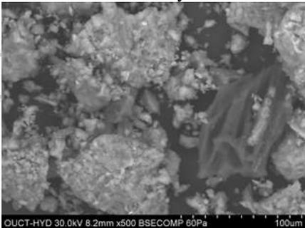
Fig. 14: SEM image of concrete with WA 10% replacement at 90 days
