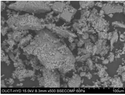
Fig. 12: SEM image of CC with WA 0% at 90 days
