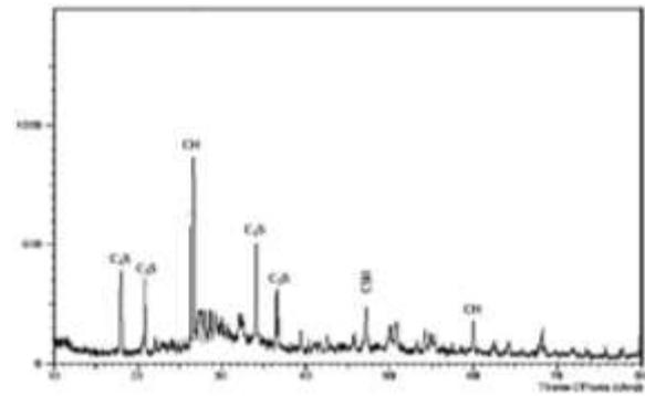
Fig. 2: XRD pattern of cement mortar (1:3) with 10% WA replacement at 28 days
