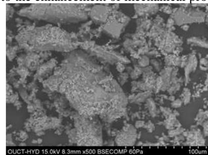
Fig. 11: SEM image of CC with WA 0% at 28 days
