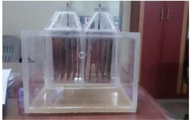
Fig. 2: Design of Electrolyser of B module
