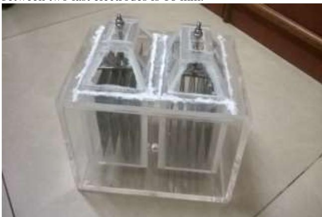
Fig. 1: Design of Electrolyser of A module
