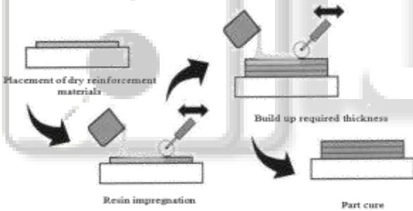
Fig. 4: Hand Lay-Up Technique
