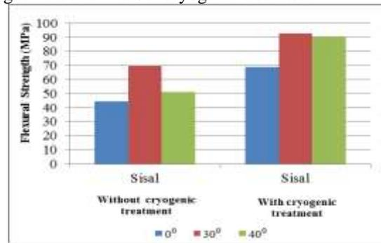
Fig. 13: Overall Comparison of flexural strength with and without cryogenic treatment.
