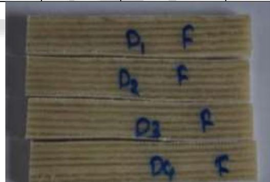
Fig. 8: Flexural Test specimens
