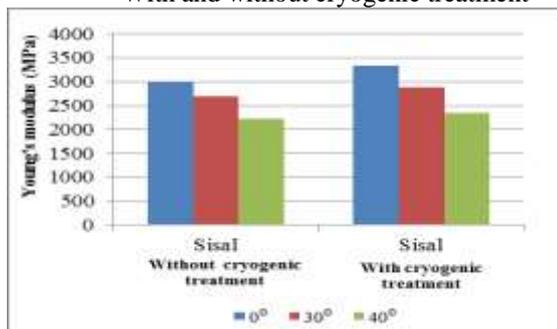
Fig. 12: Overall comparison of young's modulus with and without cryogenic treatment
