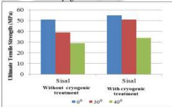
Fig. 11: Overall comparison of ultimate tensile strength With and without cryogenic treatment
