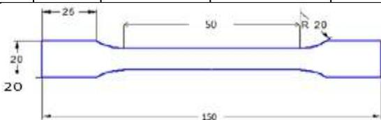
Fig. 5: Specification of tensile test specimen according to ASTM standard
