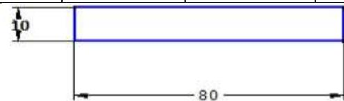
Fig. 9: Specification of impact test specimen according to ASTM standard
