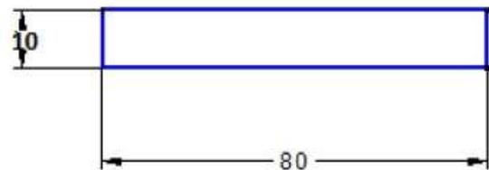
Fig. 7: Specification of flexural test specimen according to ASTM standard
