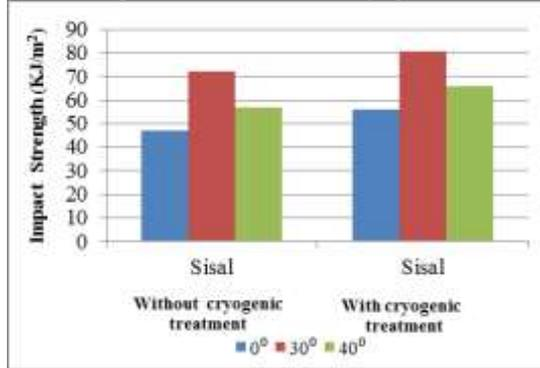
Fig. 14: Shows overall comparison of impact strength with and without cryogenic treatment.
