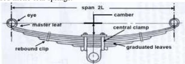
Fig. 1: Laminated semi-elliptical spring
