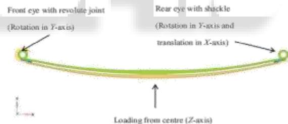
Fig. 2: Parabolic leaf spring boundary conditions.
