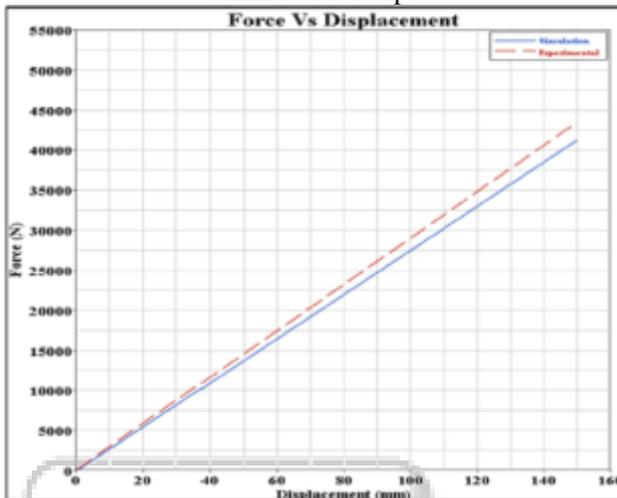
Fig. 4: Comparison of simulation versus experimental spring stiffness.
