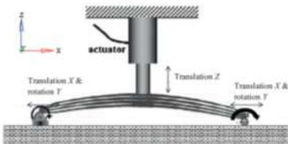
Fig. 3: Illustration of leaf spring experimental vertical stiffness test setup.
