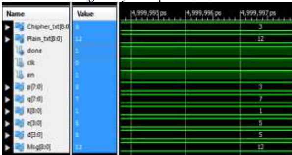
Fig. 6: Simulation result for RSA with Montgomery Multiplication
