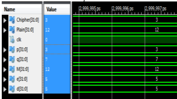
Fig. 5: Simulation result for RSA without Montgomery Multiplication
