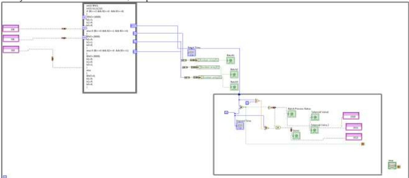
Fig. 3: Backend (block diagram) for Batch Mixing System
