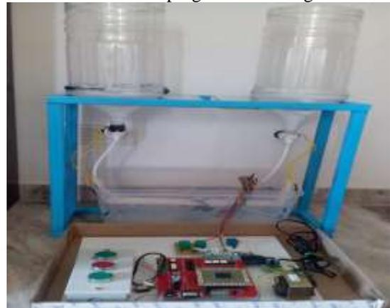
Fig. 2: Embedded PLC for Batch Mixing System
