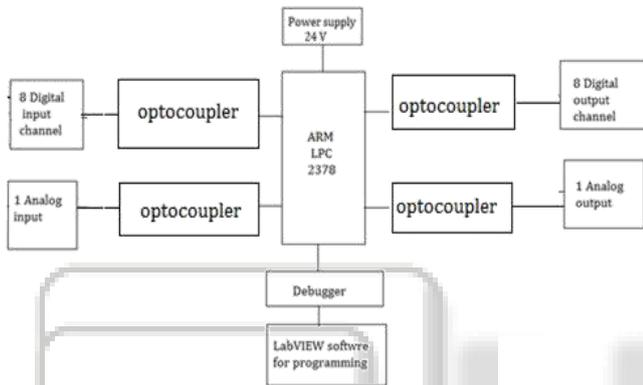
Fig. 1: Block diagram of Embedded PLC
