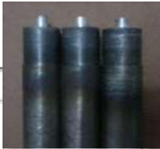
Fig. 3: Tool prepared for FSW with different pin length
