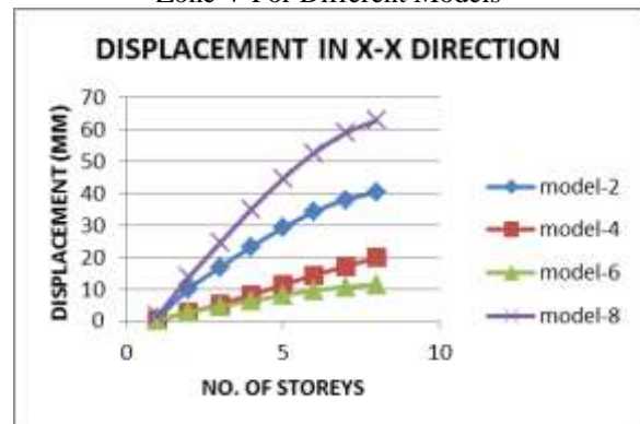
Fig. 4: Comparison of Displacement Along X Direction In Zone V For Different Models
