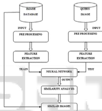
Fig. 1: block diagram for system designed
