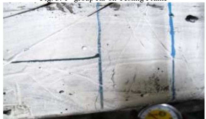
Fig. 4 Crack in Tension Zone Propagates in Upward Direction
