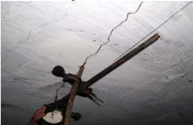
Fig. 6: crack pattern on the bottom of group RS
