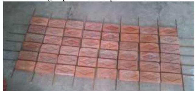
Fig. 1: Arrangement of Bricks with Reinforcement Cage
