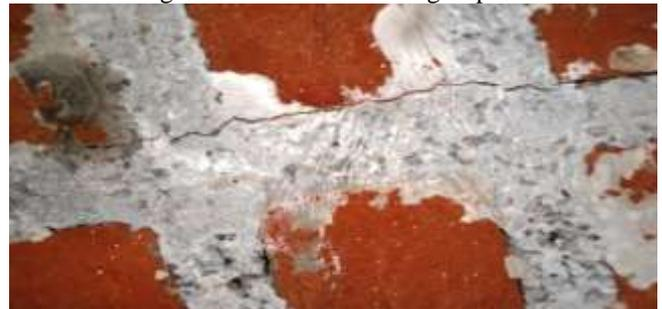
Fig. 10 crack pattern on bottom of group CS
