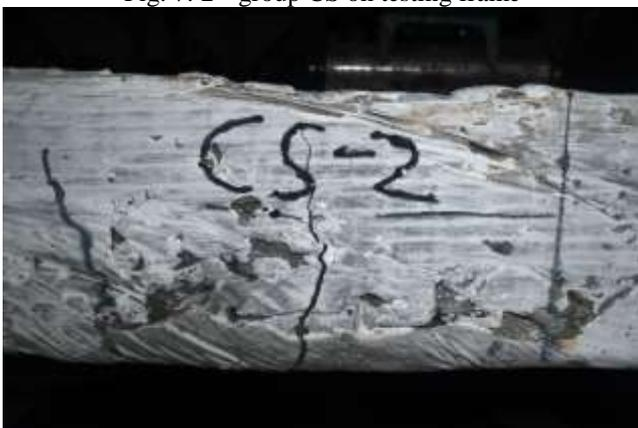
Fig. 8: Crack in Tension Zone Propagates in Upward Direction
