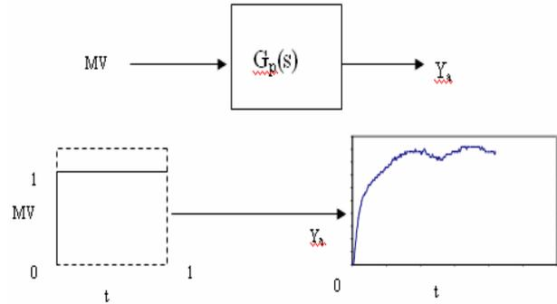
Fig. 4: Block diagram and input/output graph of open-loop test.
