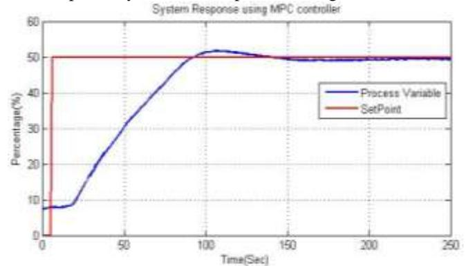
Fig. 7: System response using MPC controller for set point tracking
