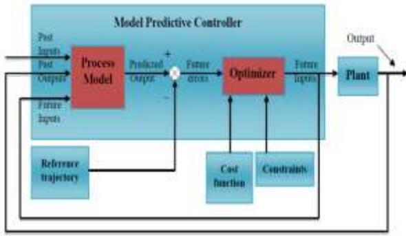
Fig. 5: Structure of Model Predictive Control.
