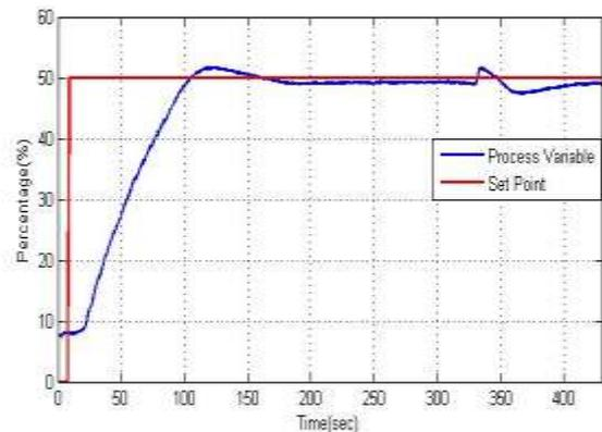
Fig. 8: System response with disturbance rejection using MPC
