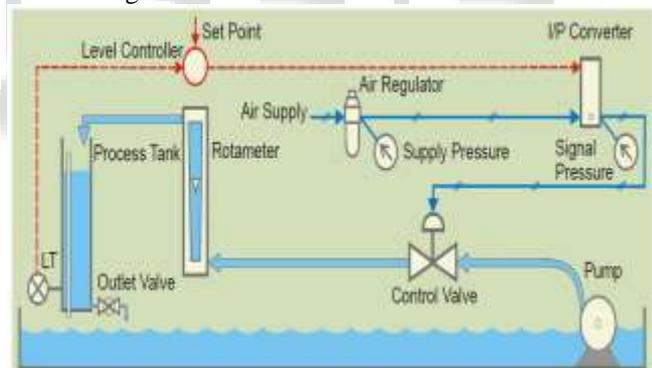
Fig. 1: P&I diagram of Liquid Level System
