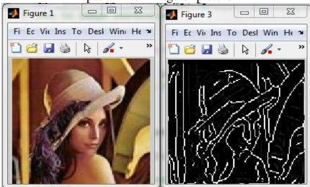
Fig. 15 Input image and block level edge detected using spatial filter image of lena
