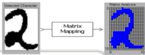
Fig. 5: Mapping numeric images onto a binary matrix
