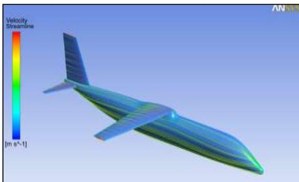
Fig. 18: Velocity streamlines over RTA Model
