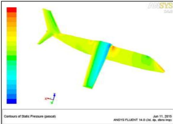
Fig. 15: Surface Pressure Contours over RTA Model at Mach number 0.5
