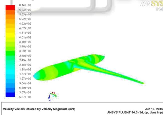
Fig. 12: Velocity Vector Colored by Velocity Magnitude.
