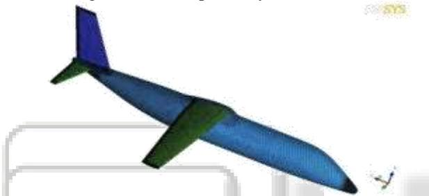
Fig. 5: Coarse Mesh on RTA Model
