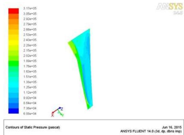
Fig. 13: Pressure Distribution on Upper Side of Wing
