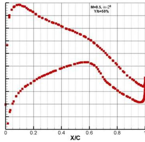
Fig. 19: Pressure coefficient distribution over wing surface at Y/b = 50%.
