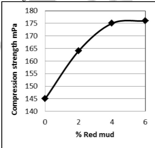
Fig. 3: Compression strength of Matrix and MMCs
