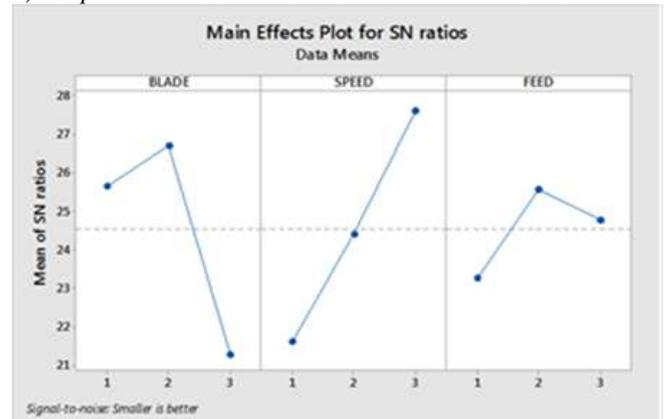
Fig. 5: Means of S/N ratio graph for tool wear
