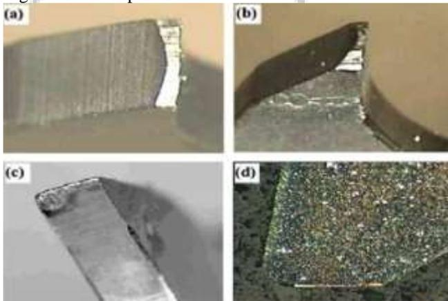
Fig. 2: Band saw wear modes: (a) flank wear (b) corner wear (c) rake face wear and (d) blunting or edge radius [2]
