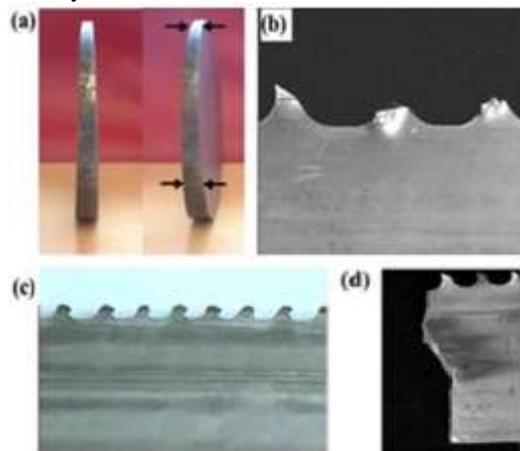
Fig. 1: Band saw failure modes: a) out of square cut b) tooth failure c) tooth wear and d) fatigue failure.<sup>[2]</sup>
