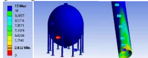
Fig 5: Safety factor of the pressure vessel
