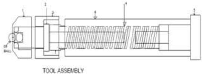
Fig. 2: Schematic diagram of the ball burnishing Tool
