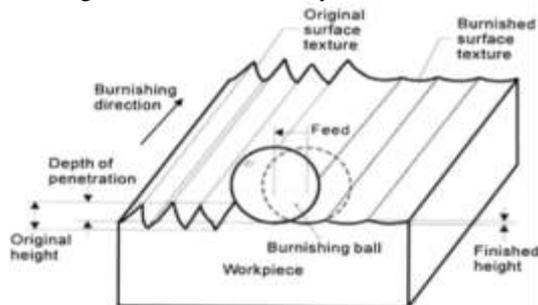
Fig. 1: Schematic diagram of the ball burnishing process
