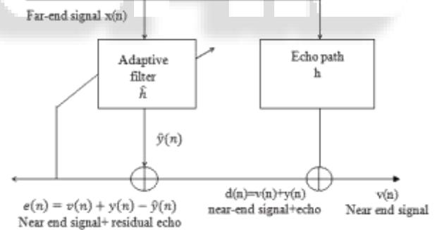
Fig. 1: Basic Model of AEC
