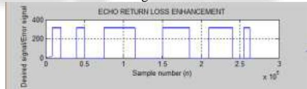
Fig. 11: ERLE of AEC with GEIGEL DTD Algorithm
