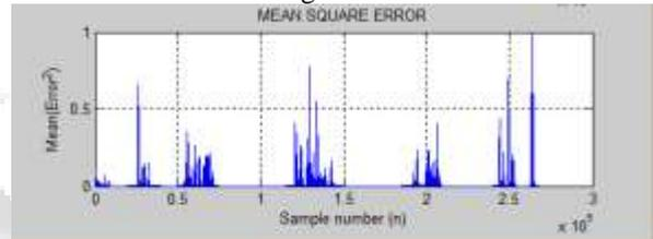
Fig. 10: Mean Square Error of AEC with GEIGEL DTD Algorithm
