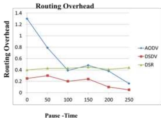
Fig. 3: Routing overhead versus pause time for AODV, DSR and DSDV (Number of node = 50, Area space = 500m x 500m)
