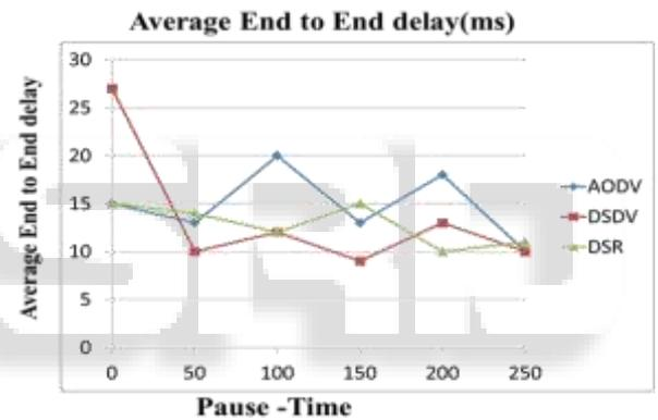
Fig. 2: Avg. end to end delay versus pause time for AODV, DSR and DSDV (Number of node = 50, Area space = 500m x 500m)
