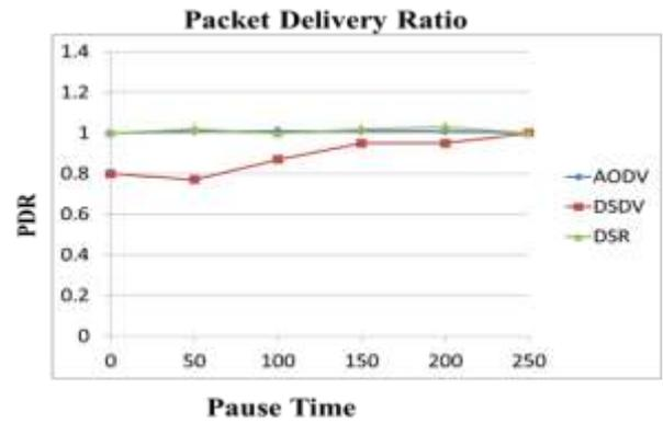
Fig. 1: Packet delivery ratio versus pause time for AODV, DSR and DSDV (Number of node = 50, Area space = 500m x 500m)
