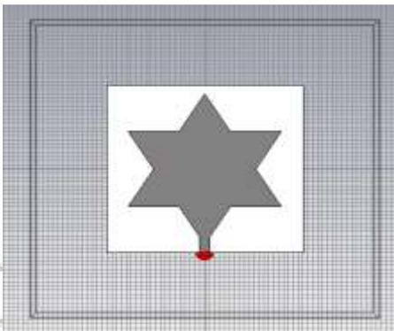
Fig. 4(a): front view of the first iteration of proposed antenna
