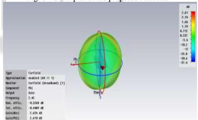
Fig. 7 Radiation patterns of the proposed antenna at 2.45GHz
