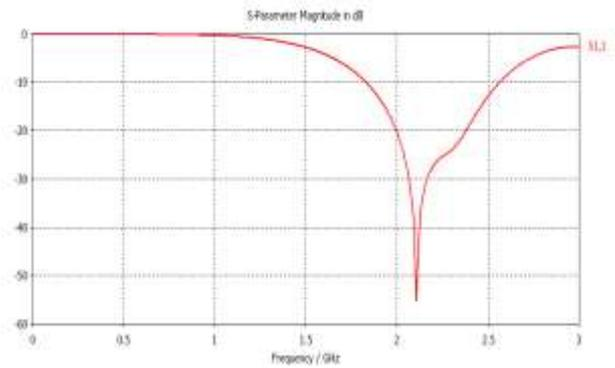
Fig. 5 (b) Return Loss plot of the proposed antenna shows the bandwidth of antenna 760MHz (1.8-2.483GHz)
