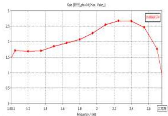
Fig. 8 Gain of the proposed Antenna Gain of the proposed antenna 1GHz to 2.7GHz which is considerable good and it is maximum at 2.3 GHz
