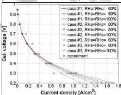
Fig. 8: Polarization curves of four different channel/rib configurations.
