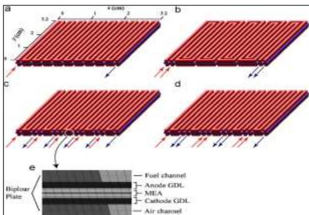
Fig. 4: The 10-cm<sup>2</sup> serpentine PEM fuel cells: (a) single channel flow-field; (b) double channel flow-field; (c) cyclic-
