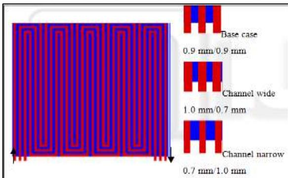
Fig. 3: 25-cm<sup>2</sup> flow-field with three different widths of channel/rib.
