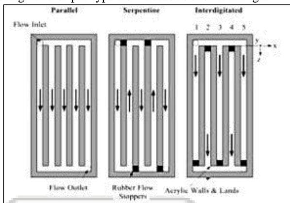
Fig. 1: Various designs of flow field plates
