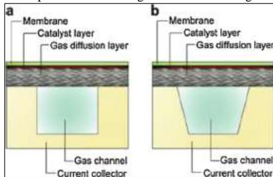
Fig. 9: Cross-sectional views of flow channel geometries. (a):rectangular; (b):trapezoidal.
