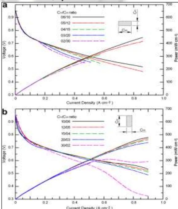
Fig. 6: Polarization curves: a) Models with horizontal cross section (06/10, 05/12, 04/15, 03/20 and 02/30); b) Models with vertical cross section (10/06, 12/05, 15/04, 20/03 and 30/02).
