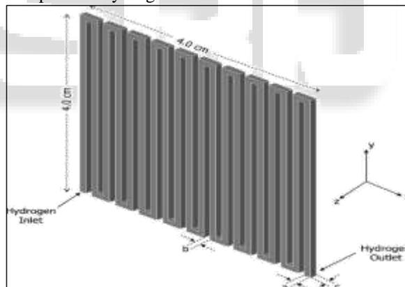
Fig. 2: Serpentine flow-field design in flow field plate showing typical dimensions for channel width (a), land width (b) and channel depth (c).
