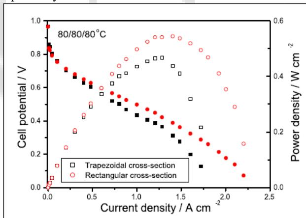
Fig. 10: Polarization and power density curves of single PEMFC
