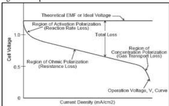
Fig. 3: Polarization curve
