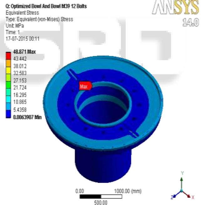
Fig 11: Von-Mises Stress (Optimized Design)
