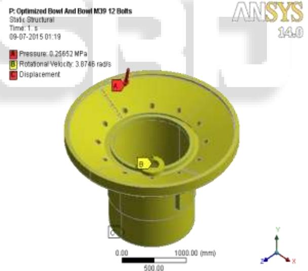
Fig 9: Boundary Conditions (Optimized Design)
