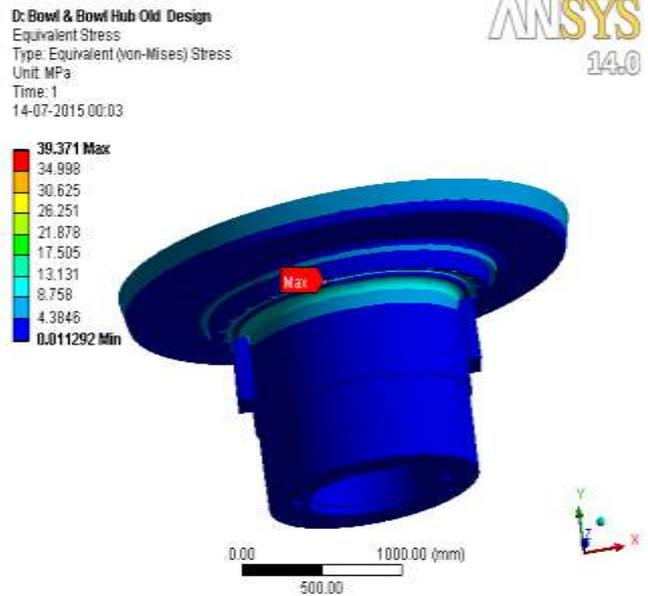
Fig 10: Von-Mises Stress (Old Design)
