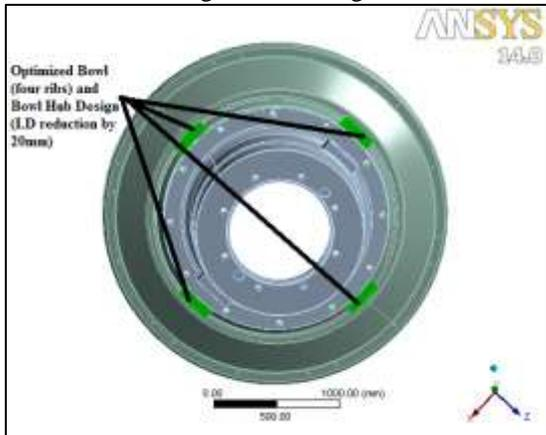
Fig 3: Optimized Bowl Design (four ribs) and Bowl Hub internal diameter reduction by 20mm
