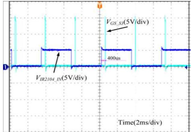
Fig. 3.2: Driving voltage of  $S_3$  and the voltage of IR2104  $S\_IN$  pin
