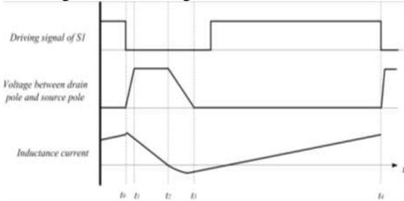
Fig. 2.2.2: Drive signal of the switch.
