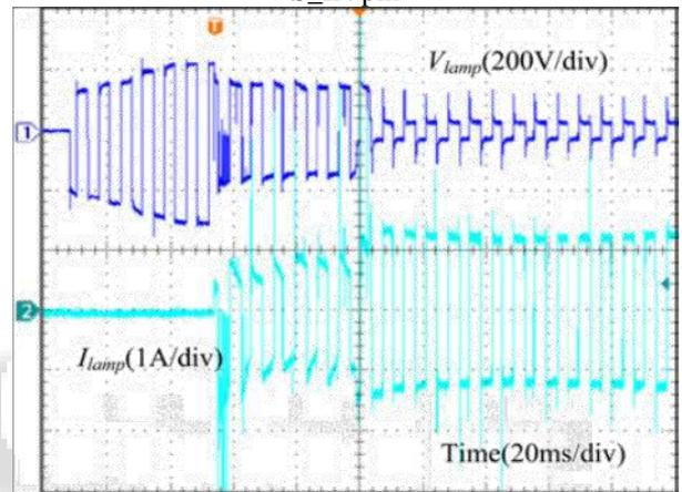
Fig. 3.3: Lamp current and lamp voltage in the igniting stage.
