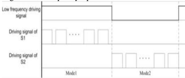
Fig. 2.1.1: Working modes of the switches.
