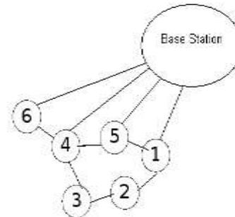
Fig. 2: Connection of different cluster heads with base stations
