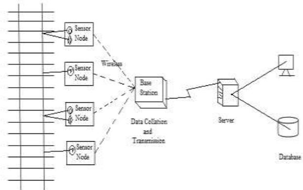
Fig. 1: Diagram shows a typical WSN setup for railway condition monitoring.
