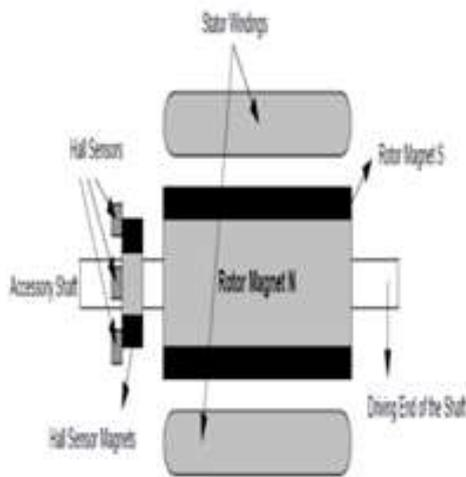
Fig. 1: Cross section view of BLDC motor
