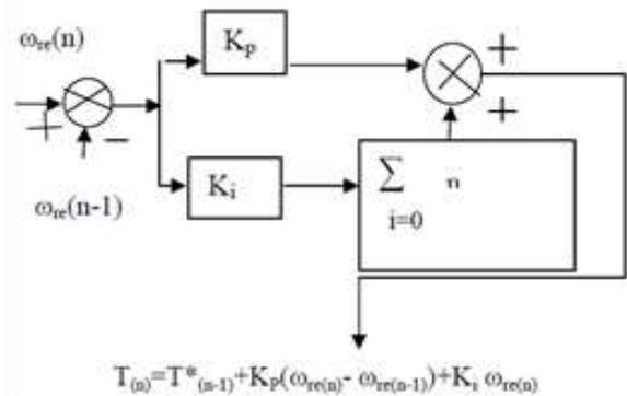
Fig. 4: Basic structure of PI controller
