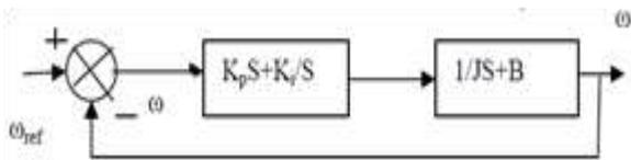
Fig. 5: Speed control using PI controller
