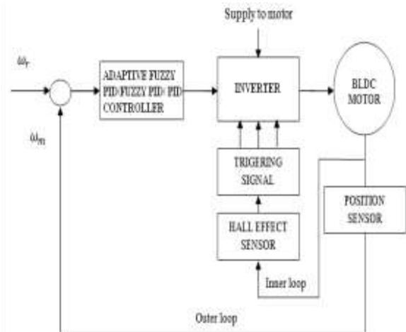
Fig. 3: Block diagram of speed control of BLDC motor
