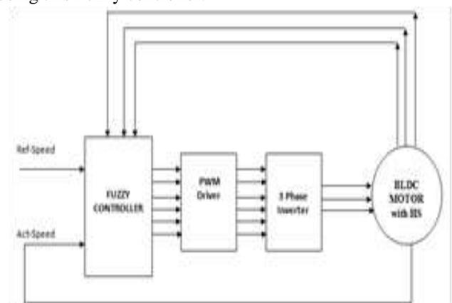
Fig. 7: Block diagram of fuzzy controlled BLDC motor drive
