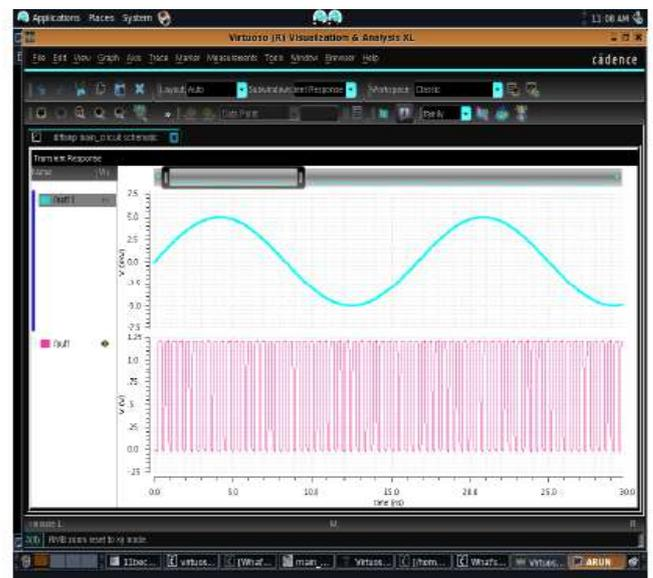
Fig 15: Waveform at the output of Phase Detector
