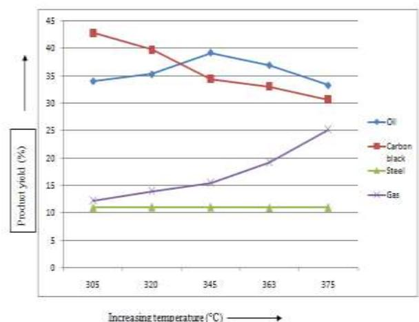
Fig. 2: End products of radial tyre
