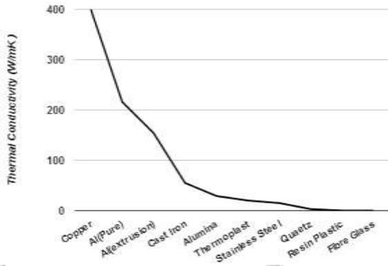
Fig. 1: Thermal Conductivities Of Various Materials.
