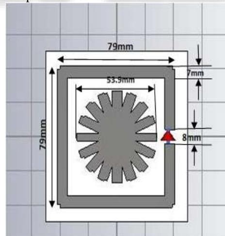
Fig. 2: Top view of cyclic loop antenna
