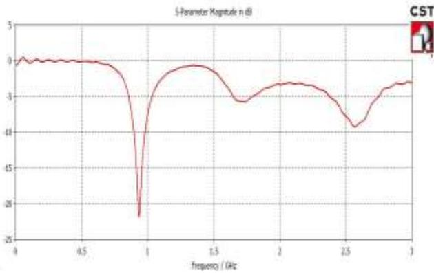
Fig. 3: Simulated reflection coefficient (S11) of proposed loop antenna
