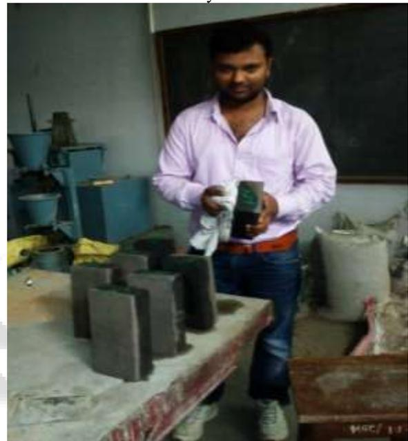
Fig. 3: Removing of water during water absorption test
