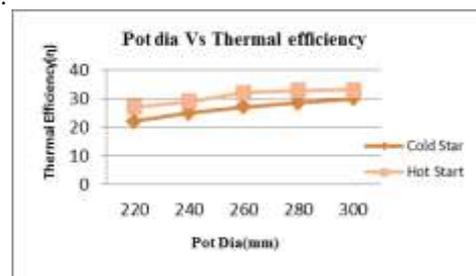
Fig-6.3: Graph between pot diameter and thermal efficiency
