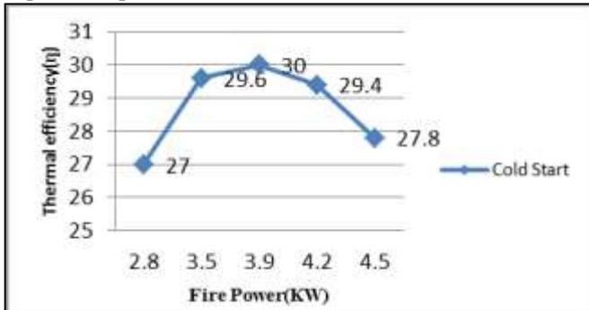
Fig-6.4.1: Graph between Fire power and Thermal efficiency for cold start
