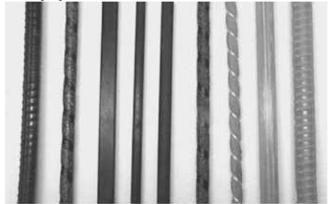
Fig. 1: Types of FRP bars and strips.
