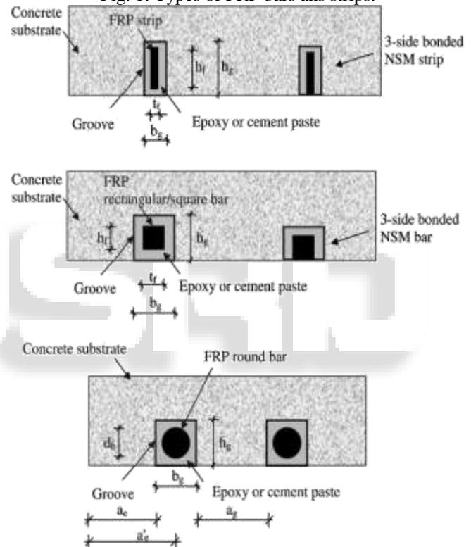
Fig. 2: Different NSM systems and nomenclature.
