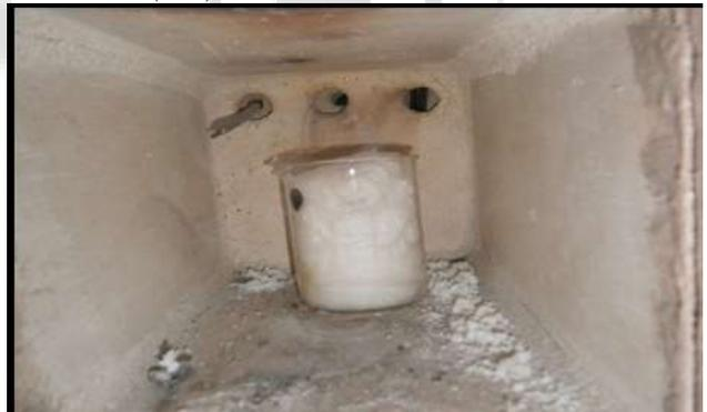
Fig. 5. a) No flame is formed when the F/O=0.4 inside the muffle furnace
