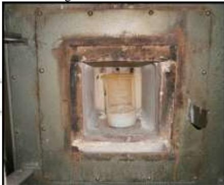
Fig. 2: Crucible inside the muffle Furnace
