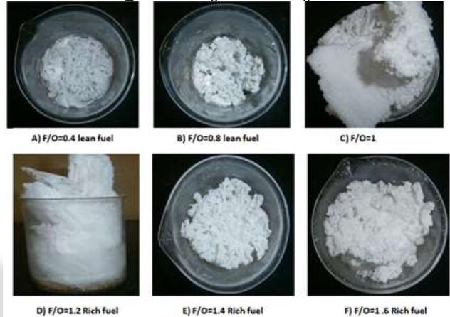
Fig. 4: Different powders formed after SCS with fuel to oxidizer (F/O) variation when urea was used as fuel.
