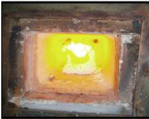
Fig. 5.c) flame is formed when the F/O=1 inside the muffle furnace
