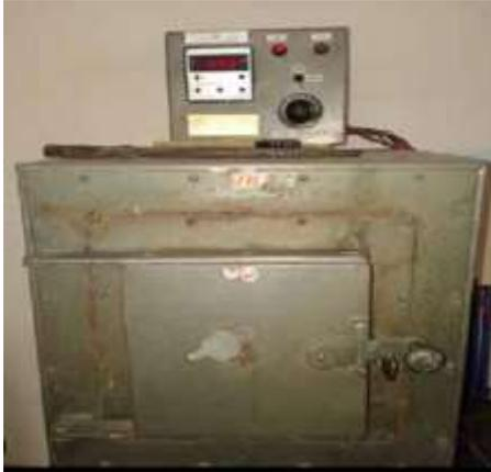
Fig. 1: Muffle furnace
