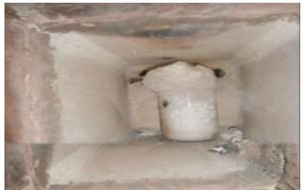
Fig. 5. b) No flame is formed when the F/O=0.8 inside the muffle furnace
