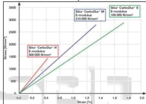
Fig. 1: Typical Stress-strain diagram
