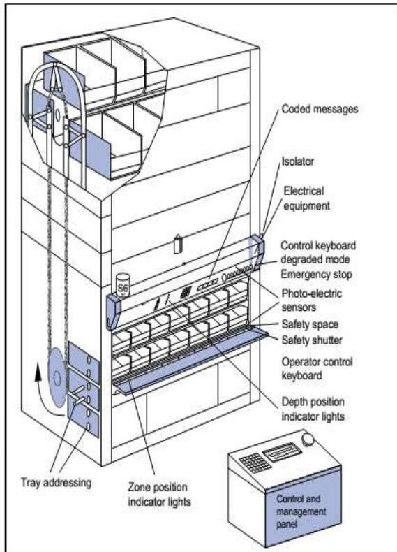
Fig. 2 Construction of Vertical Carousel Machine
