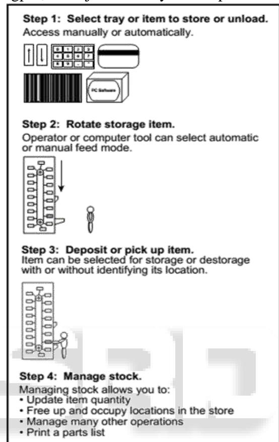
Fig. 1 Step Followed for Operation of Vertical Carousel Machine
