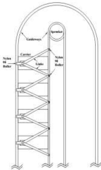
Fig. 3: Linkage mechanism in vertical carousel machine
