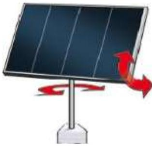
Fig. 13 Active tracking system
