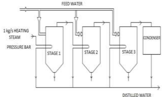
Fig. 2 Triple Effect Evaporator
