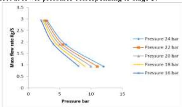
Fig.5.2 Effect of Mass Flow Rate on Inlet Pressure
