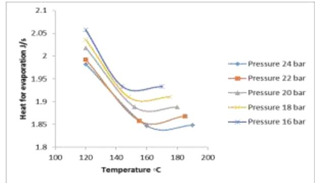
Fig.5.3 Variation of Heat for Evaporation at Different Temperatures.
