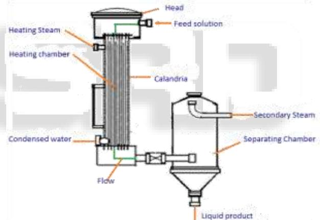
Fig. 1: Falling Film Evaporator
