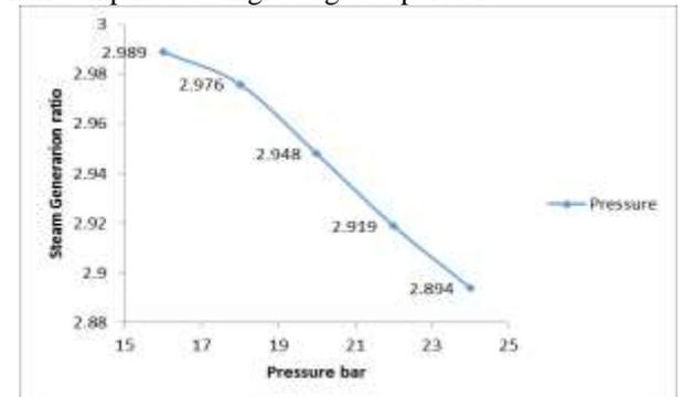
Fig: 5.5 Steam Generation rate for Different Input Pressures in Multi Effect Evaporator
