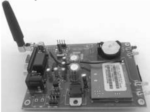
Fig. 4: GSM Modem Prototype
