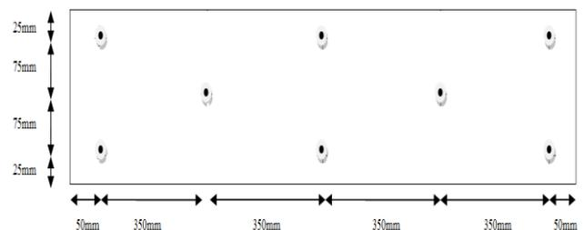
Fig.3. Position of thermocouple
