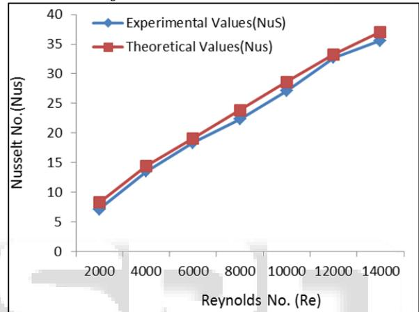
Fig. 5: Comparison of Nusselt number with experimental value and theoretical value of smooth surface.
