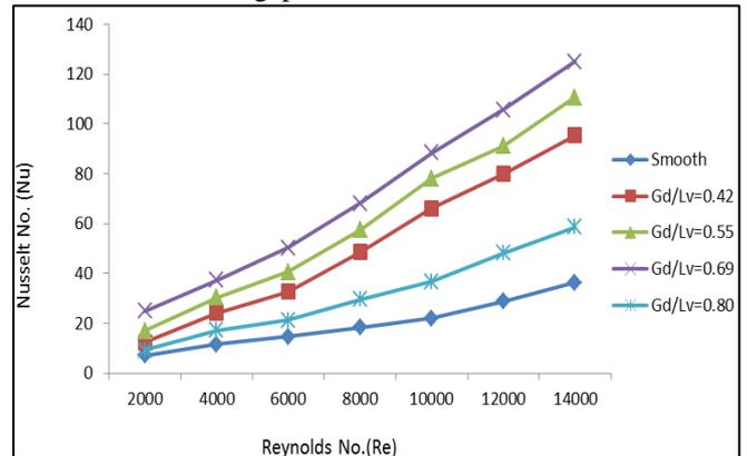
Fig. 6: Effect of relative gap distance on Nusselt number.
