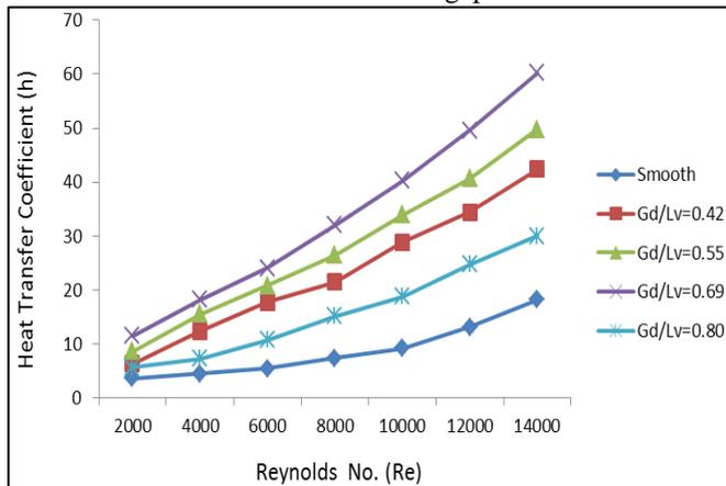
Fig. 7: Effect of relative gap distance on Heat transfer coefficient.
