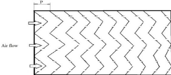
Fig. 4: Roughness Geometry
