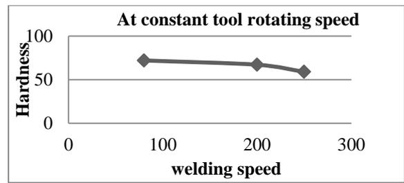
As welding speed increases temperature at the joint decreases by that hardness value also varies.
