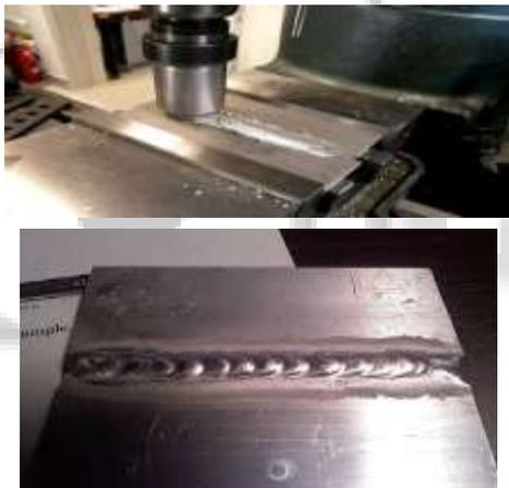
Fig. 3: layout of the plates for FSW.
