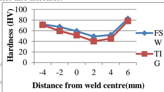
Fig 4:hardness profiles of dissimilar Al alloy AA6063 and AA7075 welded by FSW and TIG.
