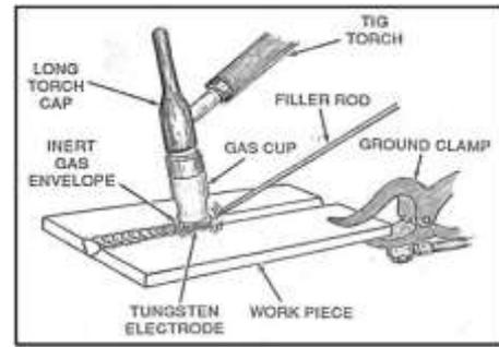
Fig. 4: schematic view of TIG welding process.
