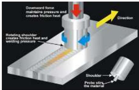
Fig. 1: schematic view of FSW process
