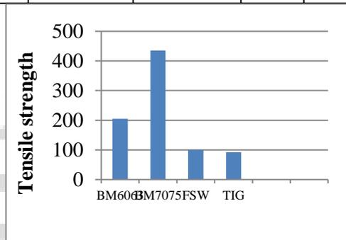
The optimum tensile strength obtained from FS welded specimens is 99.522N/mm<sup>2</sup> and from TIG welded specimens is 92N/mm<sup>2</sup>. The above graph reveals that friction stir welding gives better tensile result when compared to tungsten inert gas welding.
