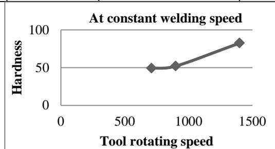
Above graph reveals that as RPM increases hardness also increases.
