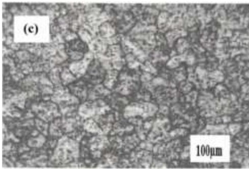
Fig. 7(c): weld centre AA6063 & AA7075
