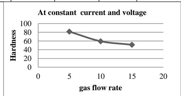
As welding gas flow rate increases temperature at the joint decreases by that hardness value also varies
