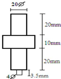
Fig. 2: geometry and dimension of stirrer tool.
